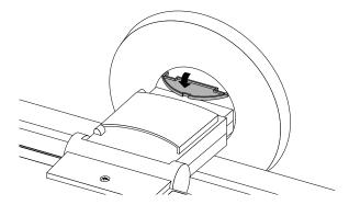
Rotate the stand base in a counterclockwise direction while holding down the protrusion, and then remove the stand base.
