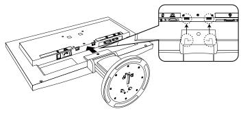
3 Prepare a screwdriver. Press the upper part of the stand against the unit and tighten the screw with the screwdriver to fix the stand to the unit.
