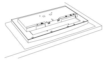
**2** Put the insertion part of the stand in the slot of the monitor.
